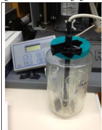
Figure 18. A wide-mouth glass jar with six film-loaded test-tubes and one test tube containing a water/salt solution to maintain the desired relative humidity, which was directly measured using a NIST-calibrated hygrometer.
